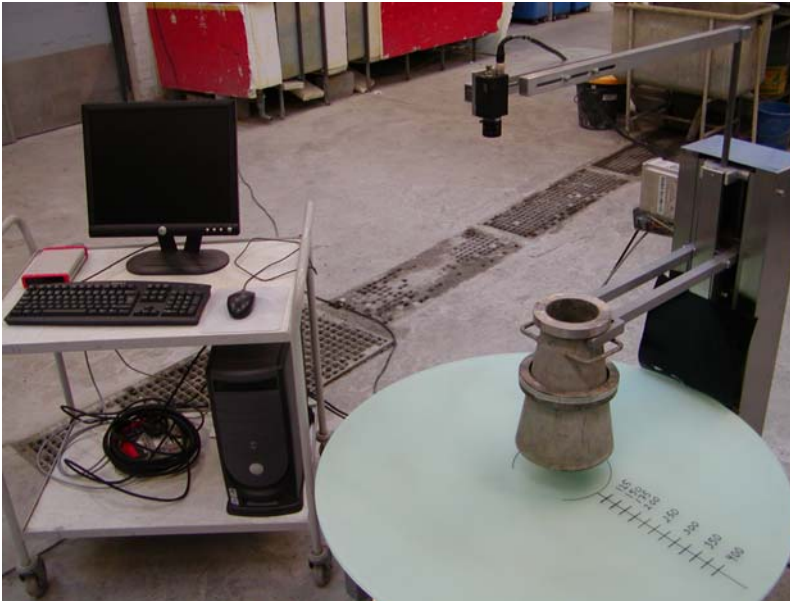
Figur 1 - 4C Auto Slump Flow systemet
